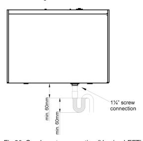
Fig 30: Condensate connection (Version LEFT)
