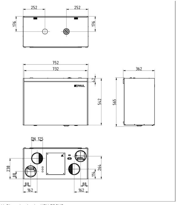
Fig 44: Dimension drawing HRU FOCUS
