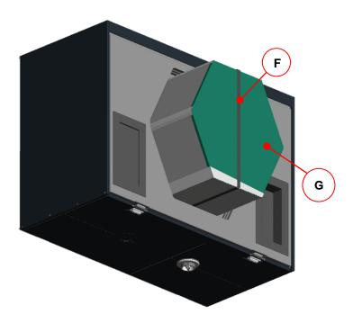
Fig 42: Remove the heat exchanger
