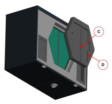
Fig 13: Dismantlement of the foam cover for filter and heat exchanger
