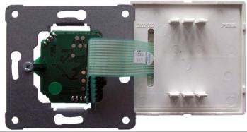
Fig 36: Adapter board with terminal X1 on an in-wall base plate; ribbon cable of the adapter board; rear panel LED key-pad (from left to right)
