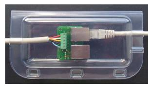
Fig 33: Casing for adapter board
