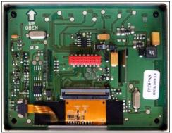
Fig 34: Adapter board with terminal X1 on an in-wall base plate; ribbon cable of the adapter board; board of the TFT touch panel (from left to right)
