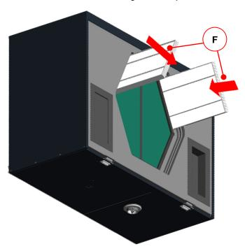
Fig 15: Install the new filter
