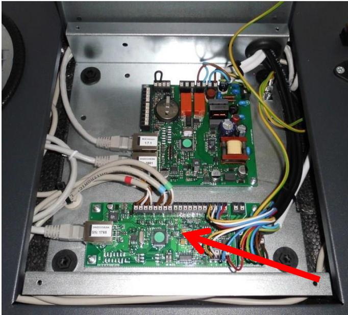
8. Install the new fan slave board in the device. Be sure to install the cables according the circuit diagram (see appendix).
