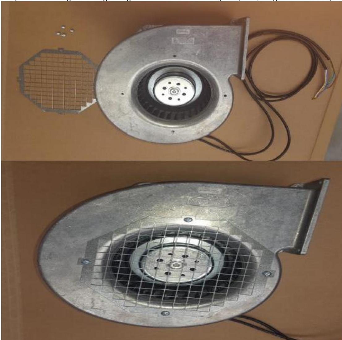
12. Plug the connector on the fan and attach him with the torx screws.
