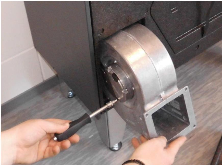
7. Insert the fan into the housing of the ventilation device. Please make sure that when you insert a new fan, the touch guard grille is installed or, if necessary, is remounted from the previous fan.
